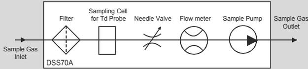
The DSS70A sampling system includes a filter to clean the dirty sample gas and a needle valve to control the sample flow rate with the flow meter. A sample pump is used to generate a sample flow from processes at ambient pressure.
