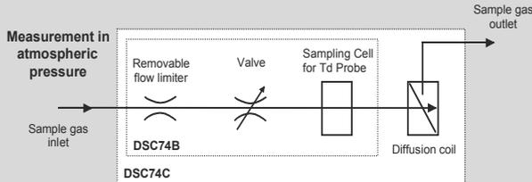
The DSC74B sampling cell enables the measurement of the sampled gas either in gas pressure up to 10 bar or in atmospheric pressure depending on the gas inlet and outlet. The DSC74C is like the DSC74B but with an additional coil to avoid back diffusion, the effect of surrounding moisture, in dew point measurements in atmospheric pressure.
